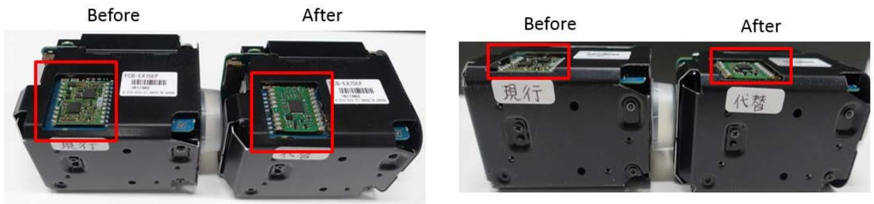
The new circuit board will be located a bit upper side, however it is not over the FCB outside surface.
